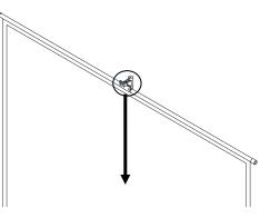
Loosen the ribbed knob on the shaft and retract the pole to its original length. Securely tighten the ribbed knob. Release the latch on the carrying handle and raise the case back to its original position and re-secure the latch.
