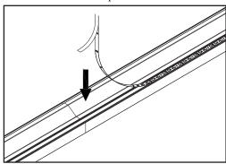
**3c.** When all the LED strips are in place, the frame should be as shown below. Make sure all of the LED strips are securely in place.
