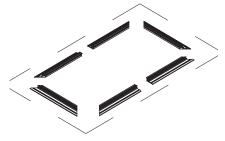
**1a.** Slide the two mounting anchors (9) into the top groove from the two ends of the frame. The anchors must be installed on the bottom frame. Please note the single small arrow which indicates the groove shown below.
