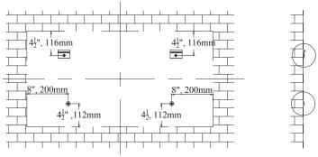
Draw a center line for your screen in the desired location. Mount the Hanging Bracket centered to your screen and 4 1/2" (116 mm) from the top of the screen. Next, mount two pairs of Mounting Plates 4 1/2" (116mm) from the bottom and 8" from the sides as shown above.
