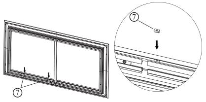
**2b.** Insert the control box screws and mount the LED Control Box (4) as shown below. Mount the box as far away from the screen material as possible, align the screws and tighten them.
