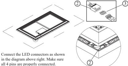
**3e.** Feed the power cord up through the holes in the frame and plug into the control box. Connect two LED connectors to the two ends of the LED strip as seen below. Feed the LED connecting cable upwards through the holes in the frame towards the LED control box.
