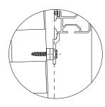
As illustrated above and below, use the provided washers underneath the Mounting Brackets or Mounting Plates to make the screen sit upright even when the wall is not completely flat.
