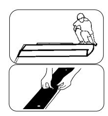
6. Take the folding legs out of the box and unfold as shown. Make sure the hinges click into place.
