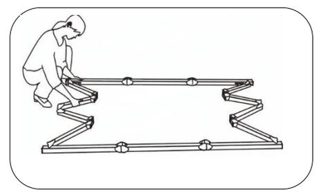
3. Make sure all 4 corners of the frame are at 90° and that the hinged support bar is straight and not bent.
