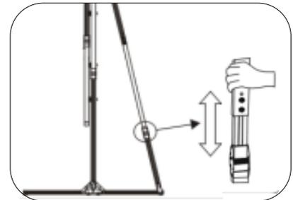
7. Lay the frame on the floor and position the legs over the sides of the frame at the desired height. Use the hand screws to loosely attach the frame. Repeat with the other leg and when in the desired position, proceed tightening both sides firmly.
