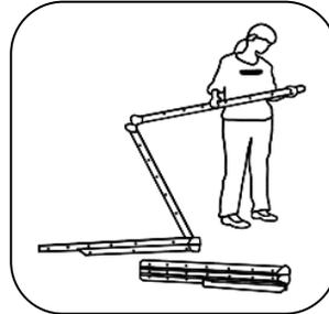
If the diagonal of your screen is 200" or greater, use the hand screws to secure the support leg to the vertical leg in an appropriate position. The support leg can be adjusted to an appropriate length. If the frame is attached to the legs higher up than the support leg, the support leg should also be attached higher up.
