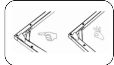
If your screen has a 200" or greater diagonal, the frame will come in 2 parts. Attach the upper frame to the lower frame and fasten 2 frames with M8x16 screws.
