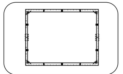
4. Take the screen fabric out of the bag and put it inside the frame next to the corner. Unfold as shown in the diagram.
