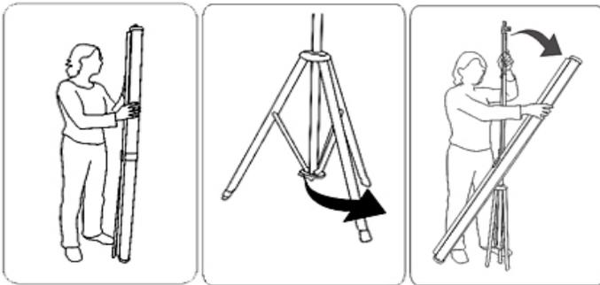
Release the latch on the carrying handle and lower the housing to the desired height and secure the latch. Loosen the ribbed knob on the shaft, extend the shaft to the desired height, and re-tighten securely.
