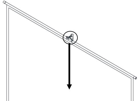
Loosen the ribbed knob on the shaft and retract the pole to its original length. Securely tighten the ribbed knob. Release the latch on the carrying handle and raise the case back to its original position and re-secure the latch.
