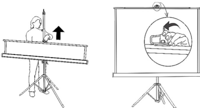
Pull the screen fabric up by using the handle on the top bar making sure it stays horizontal. Hang the handle on the suspension hook in one of the notches. The angle of the screen can be adjusted by placing the handle in different notches for keystone correction.
