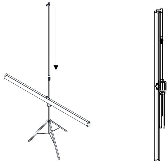
Rotate the case 90° so that it is in the vertical position and gather the tripod legs together. Loosen the ribbed knob and insert the knob on the end of the suspension hook into the slot on the housing and retighten the ribbed knob to prevent rotation when the screen is retracted.
